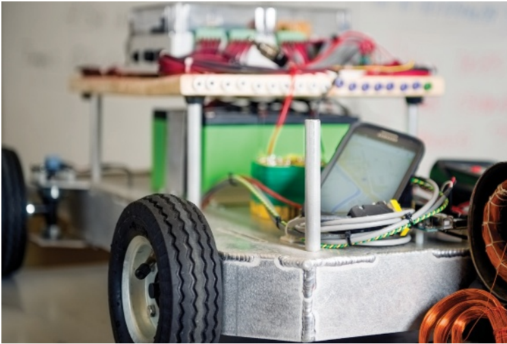
The team's technology controls the flow of energy between the supercapacitor and the battery within it, based on the car's location. It also involves optimization of the motor via modification of its winding configuration. (Photo: davidtaylorphotostudio.com).
