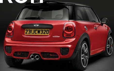
Aerodynamic improvements for the John Cooper Works include a model-specific rear apron and rear spoiler. Chromed tailpipes are centrally mounted and help provide the required aural signature.
